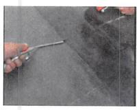
**Step 7**- Using a compressed air source, test all bonded seams using a minimum 50 p.s.i. (344.74 kPa) air supply directed through a 0.1875" (0.48 cm) nozzle held within 2.00" (5.08 cm) of the seam edge.
